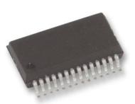
The XRT85L61 includes an on-chip crystal-less jitter attenuator with 32 bit FIFO that can either be enabled or disabled.
